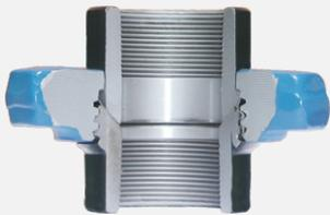
Recommended for air, water, oil, or gas service to 2000 PSI NSCWP. A union of great utility meeting most requirements in the medium pressure ranges. Precision seating surfaces assure dependable pressure seal. Standard subs are threaded for API line pipe and are Weco interchangeable. Sizes of 2" and above also available with butt weld end connections.
