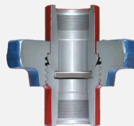
Recommended for air, water, oil, gas and mud service to 15,000 PSI NSCWP. This union has a replaceable lip-type seal ring of Buna-N specifically designed to minimize fluid flow turbulence. The lip-type ring also provides a pressure seal and protection for metal-to-metal seating surface and are recommended for manifold and truck mounting or other installations where high pressure is encountered.
