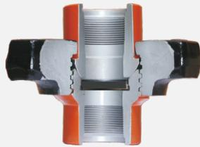
Recommended for air, water, oil, gas or mud service to 6,000 PSI NSCWP. This union has a replaceable lip-type seal ring of Buna-N specifically designed to minimize fluid flow turbulence. Lip-type ring provides a pressure seal and protection for metal-to-metal seating surfaces. Smaller and lighter than Fig. 600 unions and are recommended for manifold and truck mounting where size and weight are critical.
