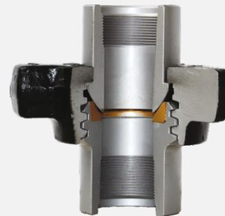
Recommended for air, oil, gas or steam service to 6,000 PSI NSCWP. Rugged and fast 2 pitch acme thread makes this the quickest union to make-up or break out (only two turns). The threaded sub is fitted with a bronze seat insert for added effectiveness in pressure sealing.
