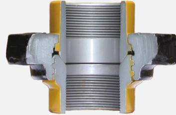
Recommended for air, water, oil, or gas service to 1,000 PSI NSCWP. Standard subs are threaded for API line pipe and are Weco interchangeable. Also available with butt weld ends.
