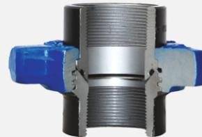
Recommended for air, water, oil or gas service to 2,000 PSI NSCWP. A Buna-N 'O' ring is mounted on the plain sub to provide an additional seal. Subs and nuts of the Fig. 206 union are interchangeable with the Fig. 200 union. Standard subs are threaded for API line pipe. Sizes of 2" and above also available with butt weld ends. connections.
