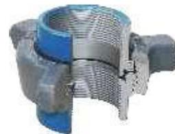
Recommended for production systems with electrolytic corrosion problems. Laminated insulating rings provide 35 million Ohms resistance across the union. O-ring in male sub provides a positive primary seal. Seal ring in female sub delivers a positive secondary seal.
