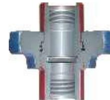
Recommended for air, water, oil, gas and mud service to 15,000 PSI NSCWP. This union has a replaceable lip-type seal ring of Buna-N specifically designed to minimize fluid flow turbulence. The lip-type ring also provides a pressure seal and protection for metal-to-metal seating surface and are recommended for manifold and truck mounting or other installations where high pressure is encountered.
