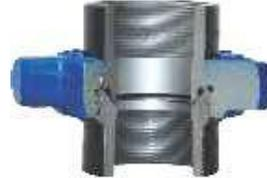
Recommended for air, water, oil or gas service to 2,000 PSI NSCWP. A Buna-N 'O' ring is mounted on the plain sub to provide an additional seal. Subs and nuts of the Fig. 206 union are interchangeable with the Fig. 200 union. Standard subs are threaded for API line pipe. Also available with butt weld end connections.
