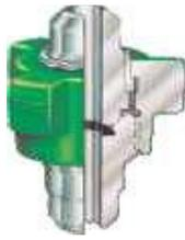
Recommended for standard service to 20,000 PSI NSCWP. Available in butt weld end connections only. Available as Fig 2202 for sour service (15,000 PSI WP).
