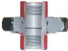
Recommended for air, water, oil, or gas service to 4,000 PSI NSCWP. Utilizes precision ball and cone seating surfaces for easy alignment and dependable pressure seal. Sizes over 4" are rated to 2,500 PSI NSCWP. Also available with a lip-type seal in 2" size only as Fig 402 and butt weld end connections.
