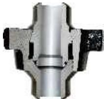
Recommended for high pressure manifolding and drilling rig use where alignment of piping components is a problem. Recommended for air, water, oil, gas or mud service to 10,000 PSI NSCWP. This union has a ball seat that allows a total of 15' (+7%) angular adjustment. An 'O' ring seal in addition to the metal-to-metal seat assures a pressure tight connection.
