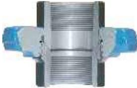
Recommended for air, water, oil, or gas service to 2000 PSI NSCWP. A union of great utility meeting most requirements in the medium pressure ranges. Precision seating surfaces assure dependable pressure seal. Standard subs are threaded for API line pipe and are Weco interchangeable. Also available with butt weld end connections.
