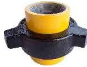
It is a flat face Union with 'O'-Ring fitted into the groove of Q the female sub. The 'O'-Ring is completely enclosed with the flat face of mating part and becomes more effective as additional pressure is applied.
