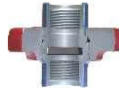
Recommended for air, water, oil, gas and mud service to 10,000 PSI NSCWP. This union has a replaceable lip-type seal ring of Buna-N specifically designed to minimize fluid flow turbulence. The lip-type ring works similarly as in the Fig. 602 union. These unions are for use on high pressure systems and trucks.
